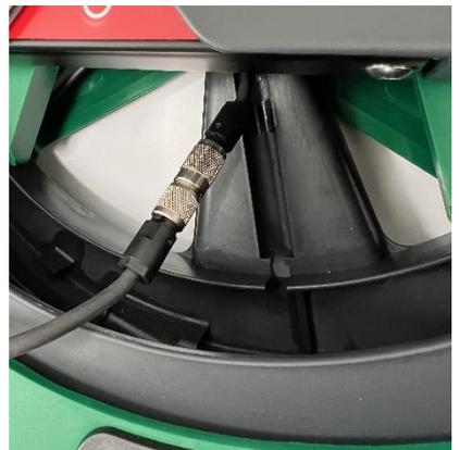
6. Unscrew the cable connector from the drum connector.
