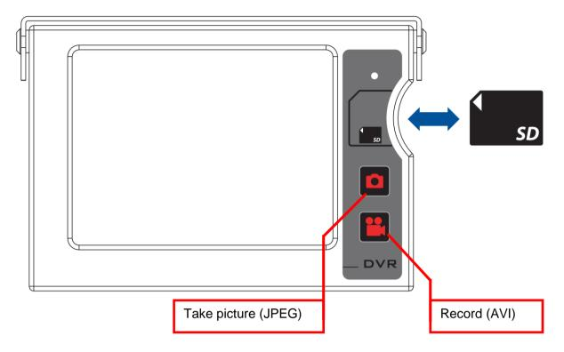
When recording starts in the upper left corner displays "REC" Data use video 2GB per hour. SD card max 16 GB.
